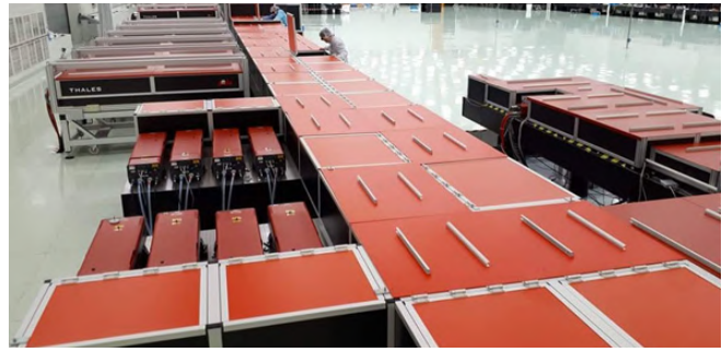
HPLS laser system installed in a dedicated 2400m 2 clean room at ELI NP, Romania
