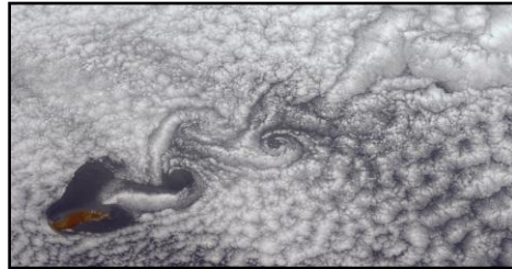
Von Karman vortex row made by the wind over the Pacific island of Guadalupe
