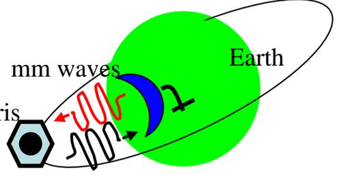
Earth-based space debris radar
