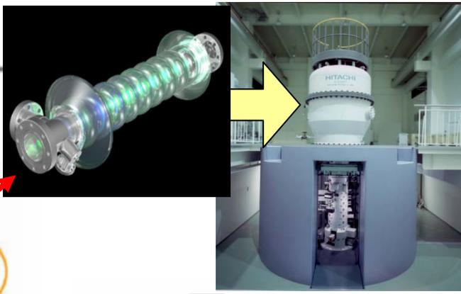
Ultra-High Voltage STEM with Superconducting RF cavity
