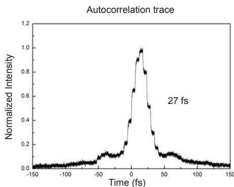
**Fig. 2** Measured autocorrelation trace of the pulse
