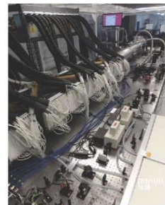
Figure 2: Liquid cooled disk amplifiers in the 600 J Apollon pump laser
