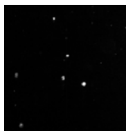
Figure 1 Image showing the damage detected on the DiPOLE system by the dark-field diagnostic
