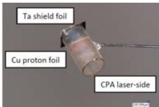
Fig. 2. Photograph of a proton tube used in EP experiments. The extent of the tube behind the Cu foil varies. For oblique incidence the foil is placed near the entrance
